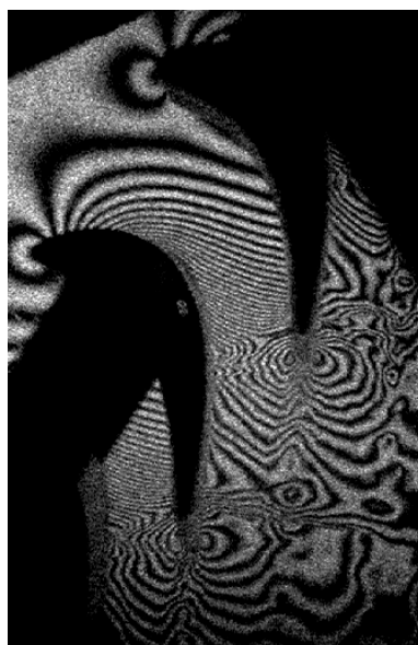
Fig.1 pulsed holographic interferogram of transonic flow at isentropic exit Mach number M=1 . The blade chord length was 58 mm.
