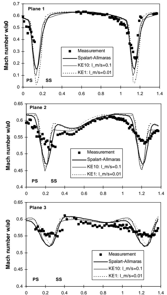
**Fig. 5: Velocity distribution in the wake flow field**
