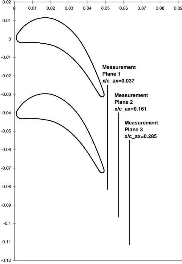
**Fig. 2: Measurement planes in the wake flow field**
