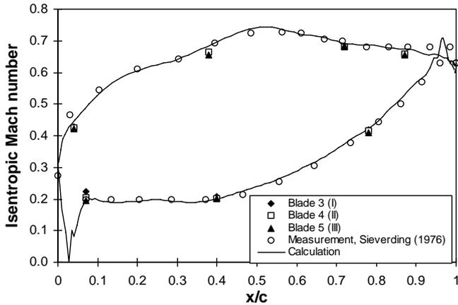
**Fig. 4: Comparison of measured and calculated isentropic Mach number distribution,  $M = 0.624$ ,  $Re=842000$**
