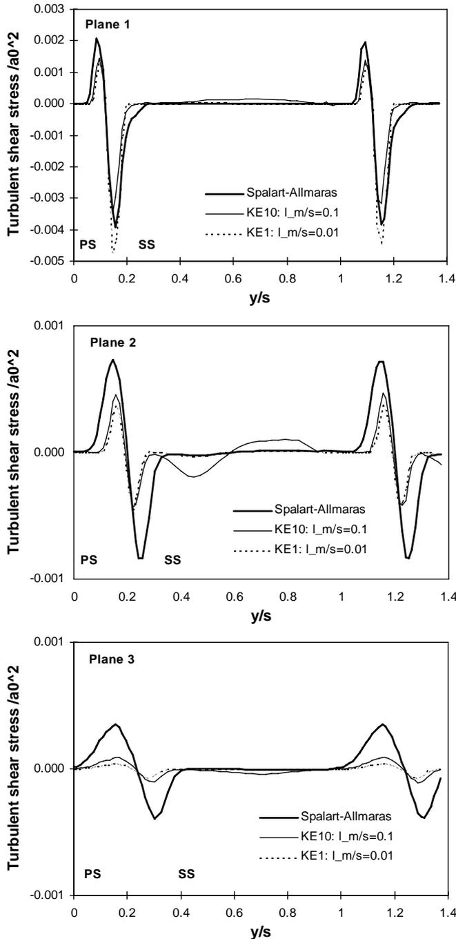
**Fig. 9: Turbulent shear stress distribution in the wake flow field**
