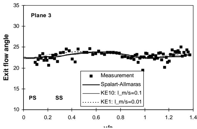
**Fig. 6: Exit flow angle in the wake flow field**
