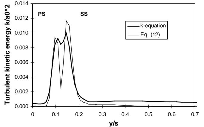
**Fig. 7: Comparison of turbulent kinetic energy predicted by k-equation and Eq. (12) for KE1, plane 1**
