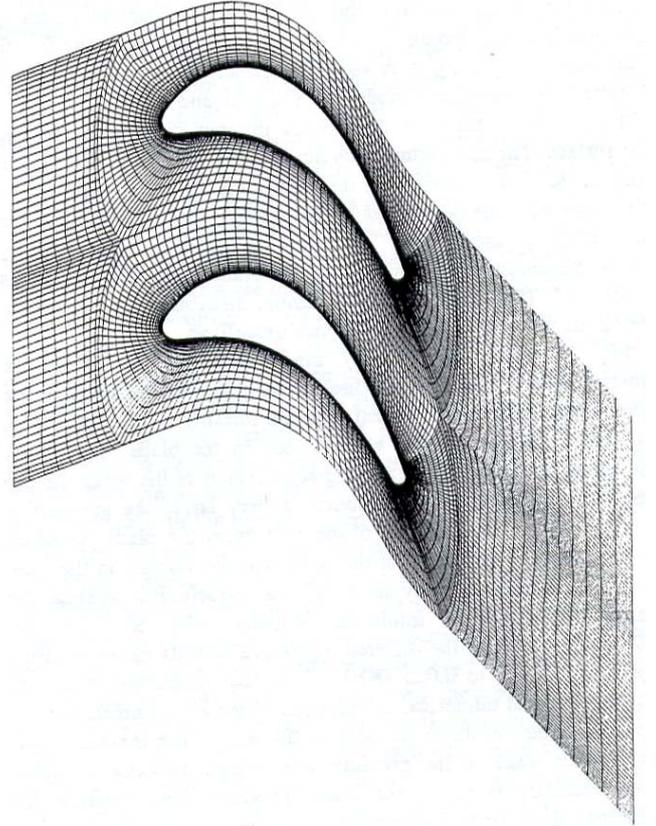
Fig. 3: Computational grid for linear turbine cascade
