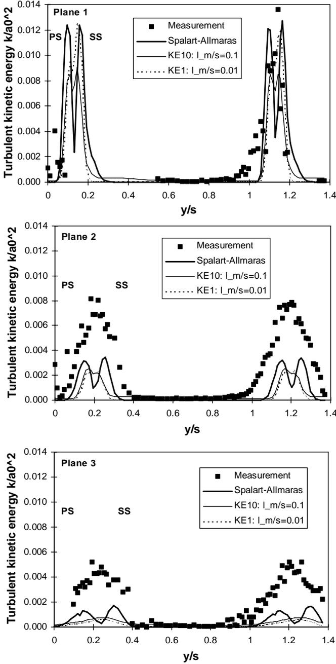
**Fig. 8: Turbulent kinetic energy distribution in the wake flow field**
