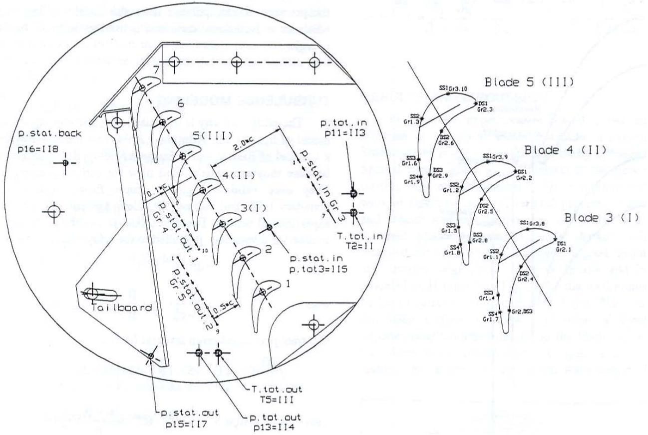
Fig. 1: Schematic of linear cascade and pressure tap location
