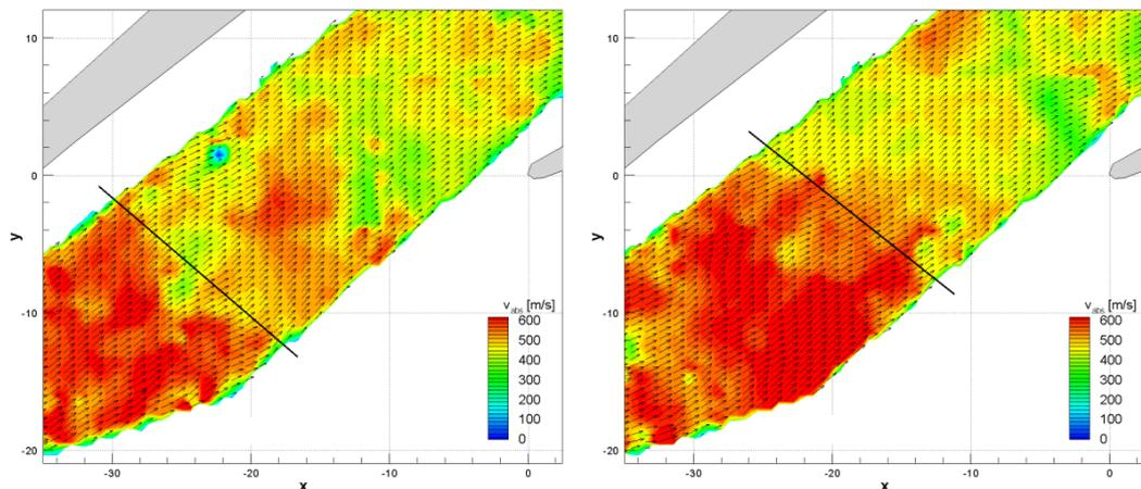
**Fig. 7** Instantaneous velocity recordings by PIV for the same rotor-vane position as shown in Fig. 6. The *line* indicates the shock position. A strong shock oscillation is observed between the *left* and the *right* image. The recording was done at the German Aerospace Center DLR, Cologne, Germany (Image courtesy of M. Voges, DLR, Cologne, Germany).
