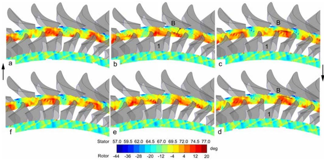
**Fig. 4 a-f** Ensemble-averaged yaw angle recorded by SPIV (see Fig. 3 for velocity). *B* indicates a stator blade, *1* a rotor blade. The single *line* in **b-d** marks the shock reflection.
