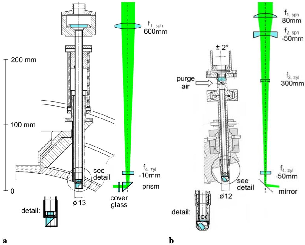
**Fig. 2** Two different light-sheet probes used for PIV. **a** shows a periscope probe used at Graz University of Technology, **b** was developed at German Aerospace Center DLR, Cologne, Germany (Image courtesy of M. Voges, DLR, Cologne, Germany).
