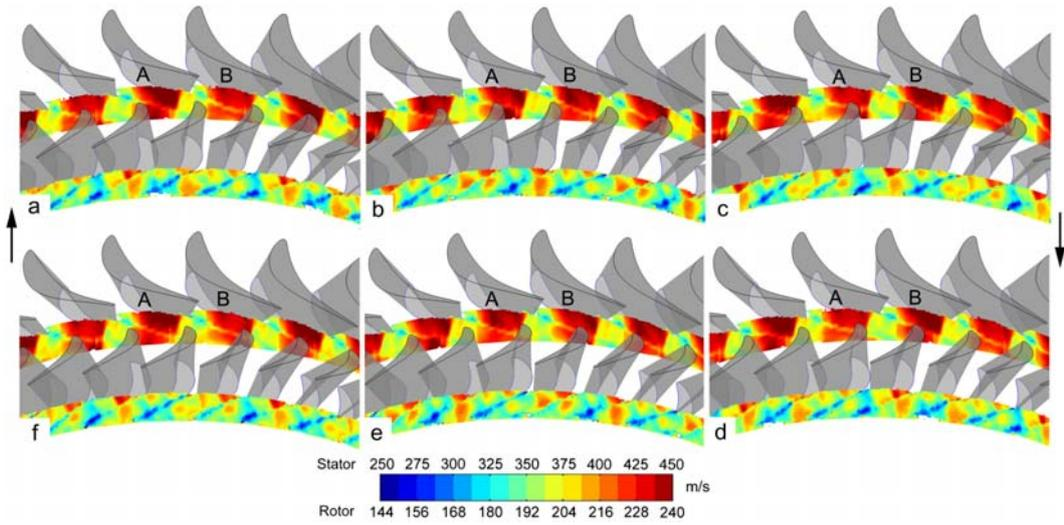
**Fig. 3 a-f** Ensemble-averaged velocity recorded by SPIV for six stator-rotor positions at 10 600 rpm, recorded in the transonic turbine shown in Fig.1. *A* and *B* indicate two stator blades.
