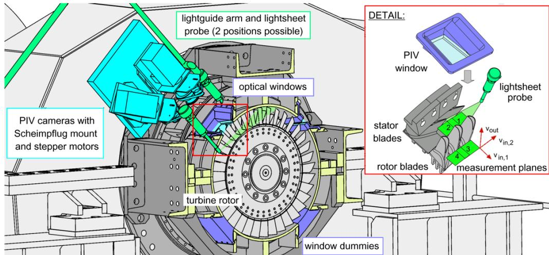
**Fig. 1** Experimental setup for SPIV at the transonic test turbine facility (TTTF) at Graz University of Technology (one-stage configuration). The exhaust part was cut off for better visibility. The *detailed view* shows the two light-sheets used and the in-plane and out-of-plane components recorded by SPIV,  $v_{in}$  and  $v_{out}$ . The optical window is a plane-concave quartz glass for the PIV (upper left window) and a plane quartz glass for laser Doppler velocimetry (upper right window).
