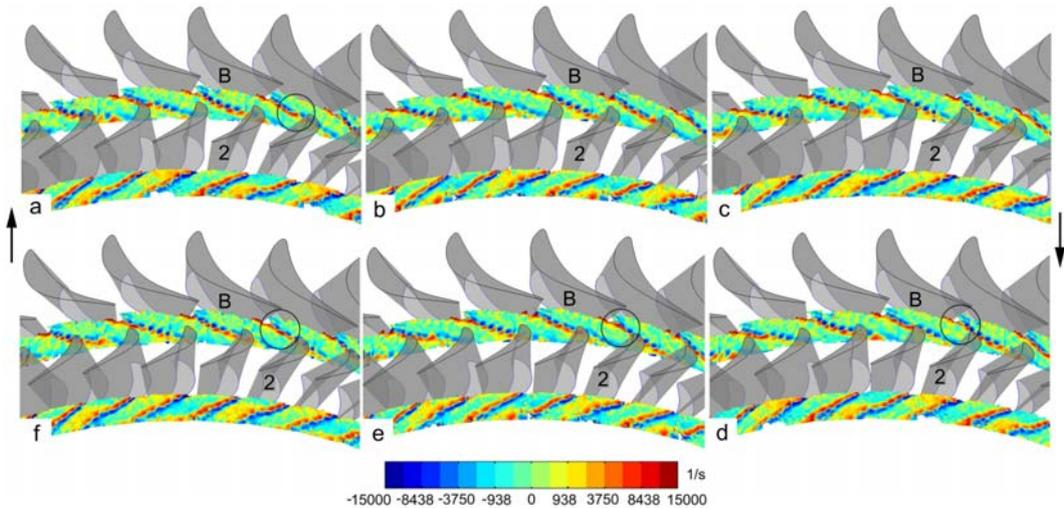
**Fig. 5 a-f** Ensemble-averaged vorticity recorded by SPIV (see Fig. 3 for velocity). *B* indicates a stator blade, *2* a rotor blade. The circles in **d, e, f, a** mark vortex shedding enforced by the shock reflection in Figs. 4b-d. Behind blade 2 vortex-vortex interference is visible in **a-f**.
