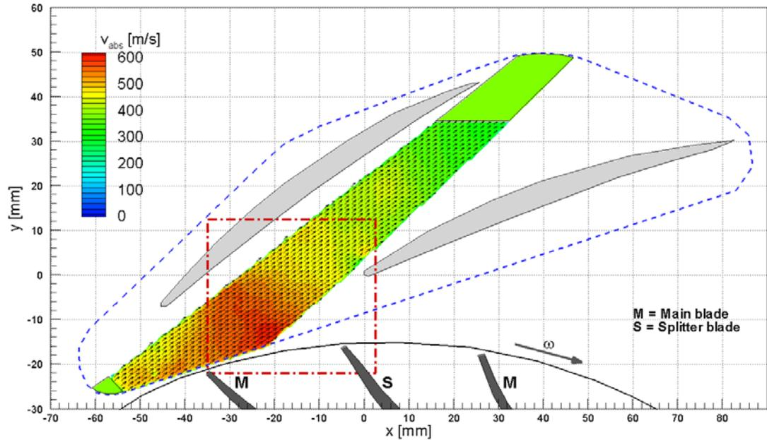
**Fig. 6** Ensemble averaged velocity recorded by PIV in the diffuser passage of a transonic centrifugal compressor at 50 000 rpm for the rotor position shown. The *dashed blue line* indicates the window section. The recording was done at the German Aerospace Center DLR, Cologne, Germany (image courtesy of M. Voges, DLR, Cologne, Germany).
