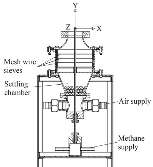
Figure 1: Cross-section of the diffusion burner used for the investigation of the density fluctuations in the methane-jet flame.
