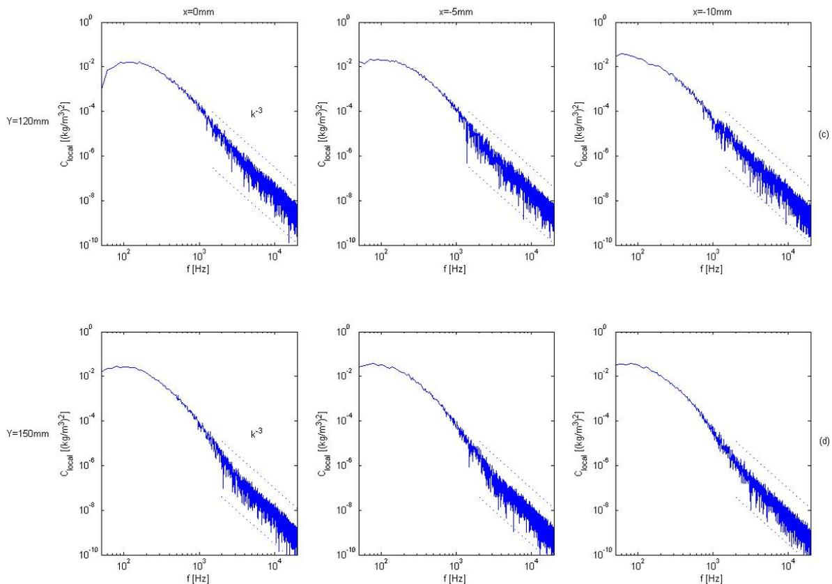
Figure 4(b), (c): Spectra of local density fluctuations at  $Y=120\text{mm}$  and  $Y=150\text{mm}$ . Dashed lines represent an exponent of  $-3$ .
