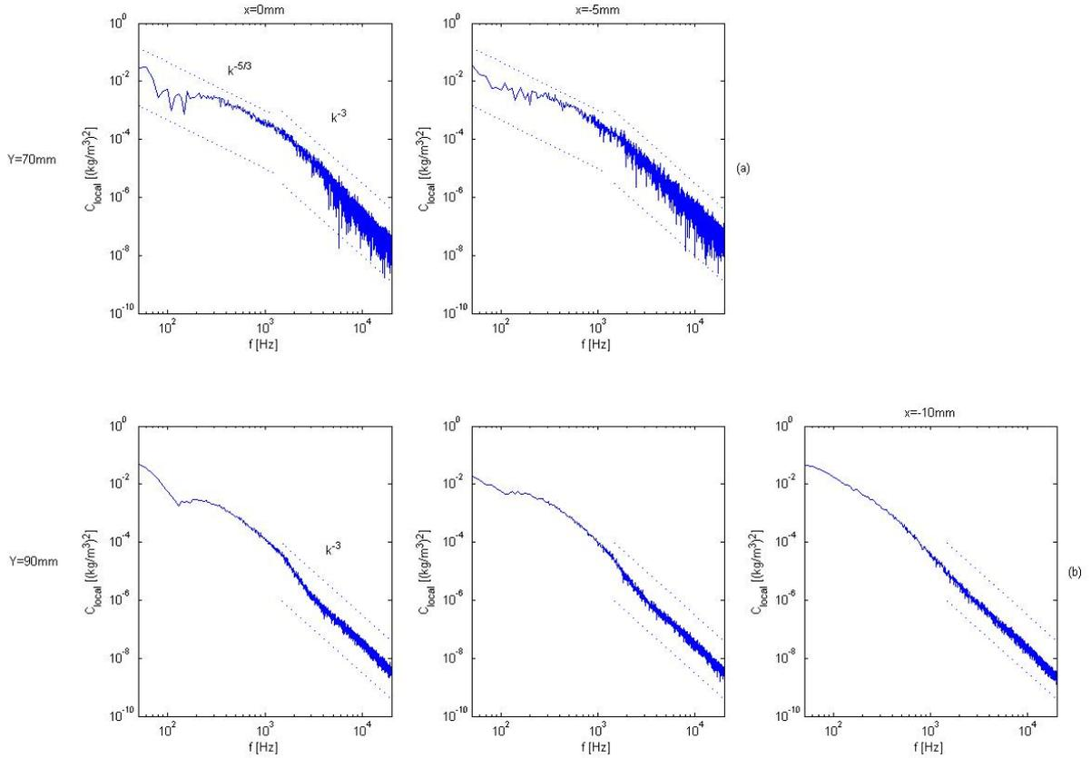
Figure 4(a), (b): Spectra of local density fluctuations at  $Y=70mm$  and  $Y=90mm$ . (a) Local spectra of the non-reactive methane-jet at  $x=0mm$  and  $x=5mm$ . Position  $x=-10mm$  is outside the methane-jet and therefore not plotted. Dashed lines represent the power law exponent  $-5/3$  or  $-3$ . (b) Local spectra of density fluctuations in the flame. Dashed lines show a decline with exponent  $-3$ .
