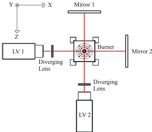
Figure 2: Principal setup of the LV for the investigation of density fluctuations in the methane-jet flame.
