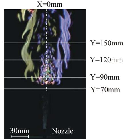
Figure 3: Color-Schlieren-visualization of the methane-jet flame. Layers for LV measurements are marked according to the coordinate-system in Figure 1.
