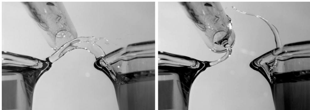
**Fig.11** Deflection of the floating water bridge in the vicinity of a charged glass rod.
