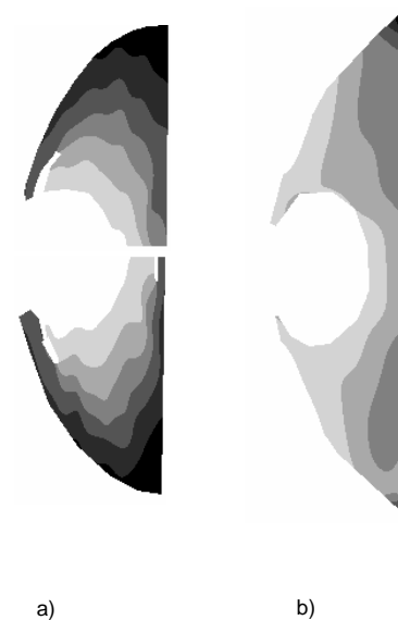
FIG 10. Pressure distribution inside the chamber for a) circular shaped and b) chamber with straighten edges. Light areas indicate high pressure zones. Stagnation pressure in the metallic pipe feeding the chamber had been 2 bar in both cases.
