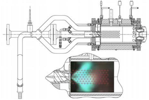
Fig. 5: LV setup (detail view: measurement points).
