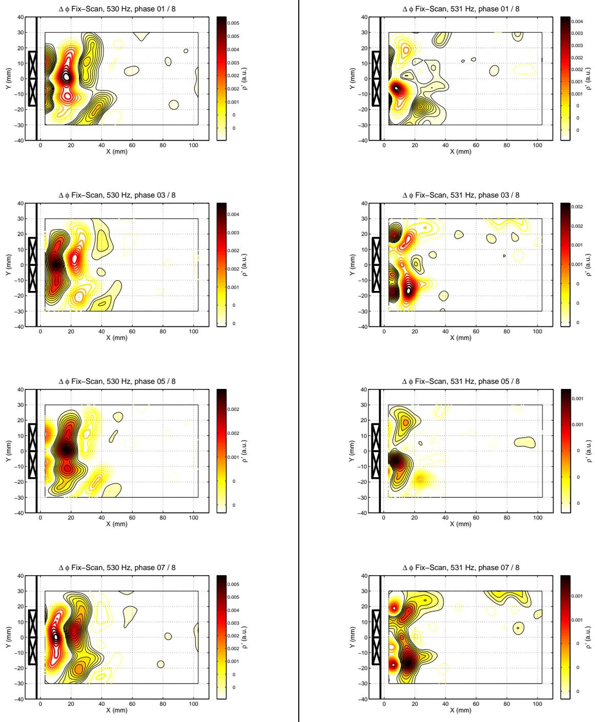
Fig. 10: Density fluctuation measurement performed with LV on a pulsed flame in closed-jet conditions (pulsation frequency at 540Hz – 4 phases are represented at 0,  $\pi/2$ ,  $\pi$ ,  $3/4\pi$ ), the filled contours represent a positive density fluctuation and the light contours negative ones, the color represents the intensity); left: atmospheric conditions, right: intermediate pressure at 2,0bar inside the combustor
