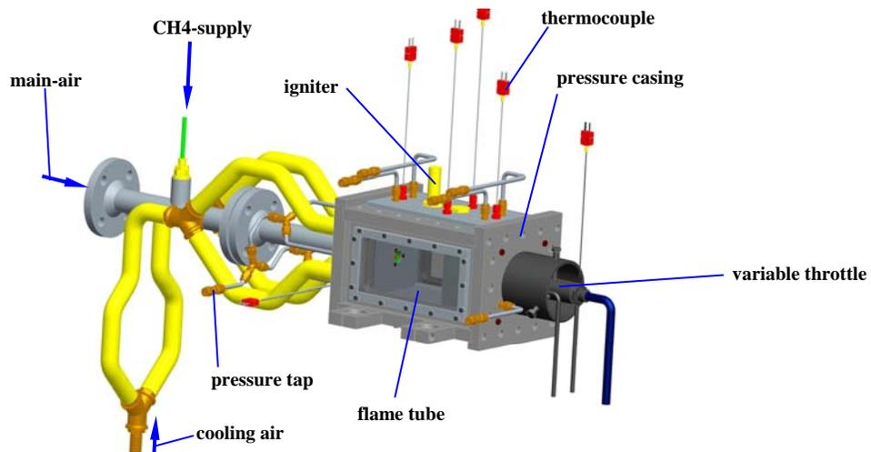
Fig. 3: Intermediate pressure combustor with air and methane supplies, variable throttle, instrumentation and optical accesses.
