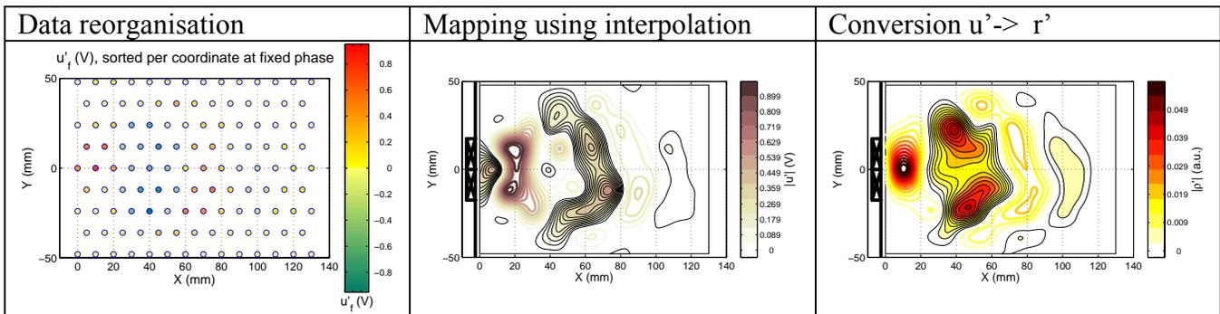
Fig. 7: Mapping process. Left: sorting of the measurements per grid point at a fixed phase. Middle: linear interpolation of  $u'$ . Right: process of  $\rho'$  map. Full contours: positive fluctuation. Line contours: negative fluctuation.
