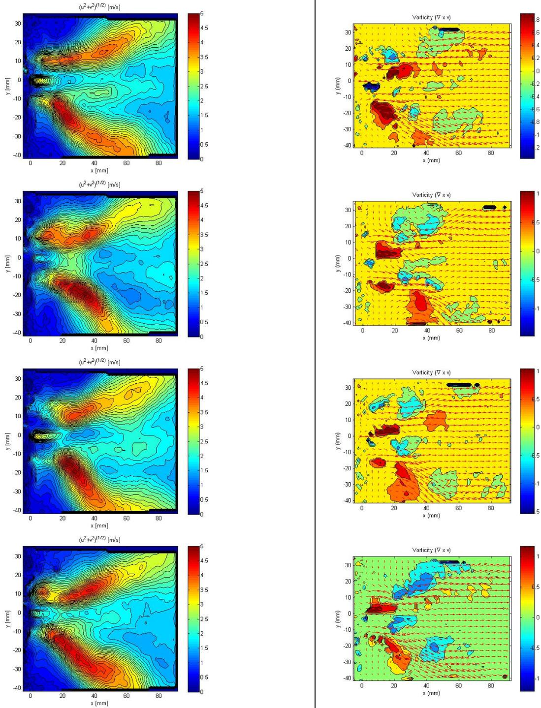
Fig. 9: Analysis of the pulsed jet dynamics (isothermal case, free jet - 4 phases 0,  $\pi/2$ ,  $\pi$  and  $3/4\pi$  are representing one cycle of operation at 33Hz); left: normalized velocity; right: vortical field analysis, where the main structures are computed based on a rotational of the velocity field
