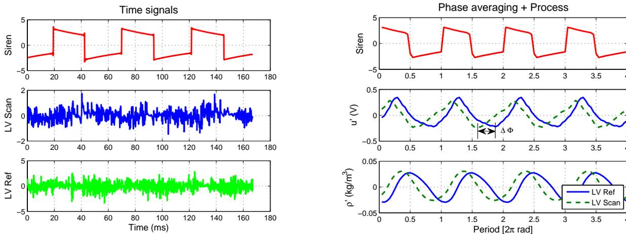
Fig. 6: Left: Time signal acquisition of the reference (siren). Right: LV signal, and phase-averaging post process.
