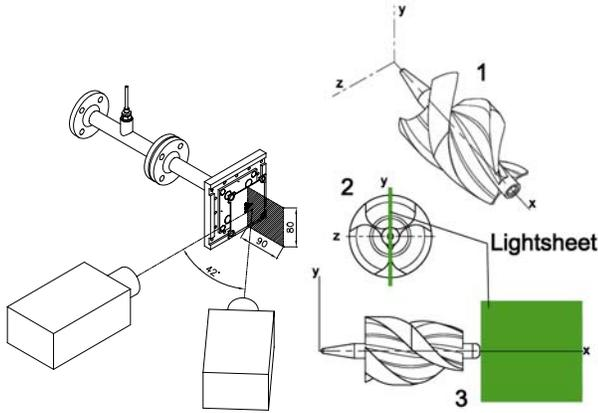
Fig. 4: PIV measurement setup; left: camera setup; right: 1. coordinate system, 2. front view, 3. side view
