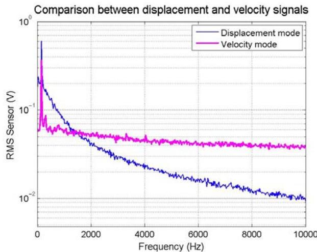
Fig. 8: Comparison between the displacement mode and the velocity mode
