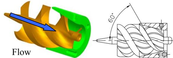
Fig. 2: Axial swirler with swirl angle  $60^\circ$  and Venturi tube; left: 3D-view; right: side view.
